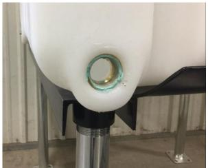
7. Install 1" Brass Spring Release Valve (P/N: RTT-4001) directly into bottom tank drain port. Install additional Valves into Elbow Kits on Stand. Be sure to support the Elbow Kit so as not to put unnecessary pressure on the Elbow Kit Bolt.
